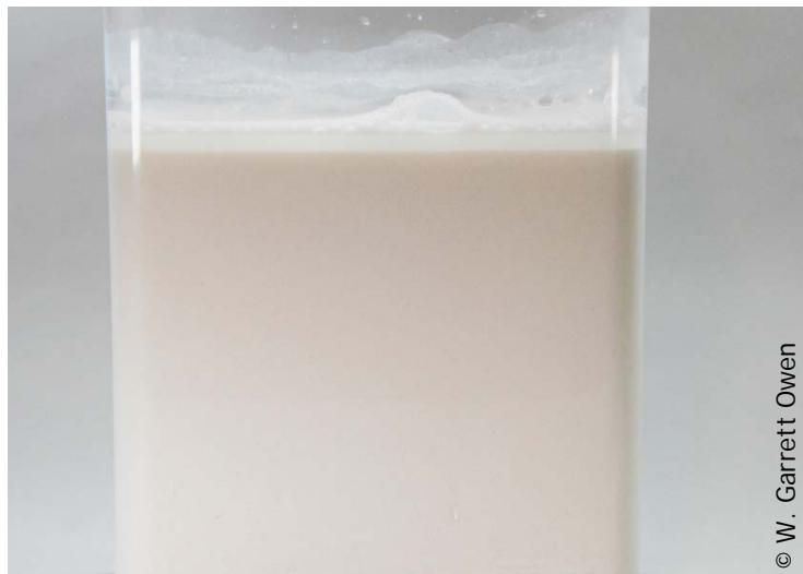
Figure 2. Mix 1 pound of hydrated lime in 3 to 5 gallons of WARM water. Photo by: W. Garrett Owen
