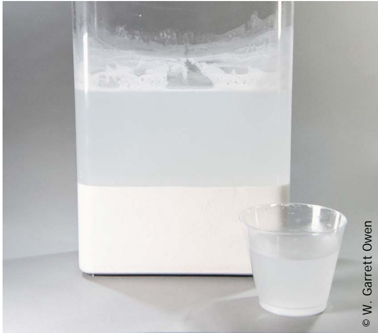
Figure 5. Decant or carefully pour the clear liquid without disturbing the insoluble solid portion. Photo by: W. Garrett Owen
