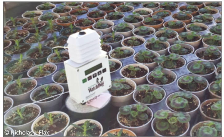
Figure 3. Data loggers equipped quantum sensors can monitor and record average instantaneous light intensity and daily light integral (DLI). Certain hand-held meters can be used in a similar manner, and many greenhouse environment controllers have integrated PAR sensors to track light in multiples bays at once.
