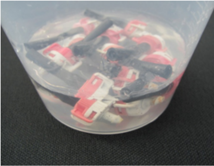
Figure 3. Irrigation emitters with biological biofilm build-up should be soaked in a dilute bleach solution. Photo: Courtesy of Cleanwater3.org.
