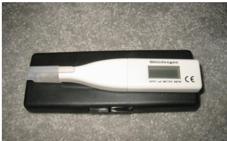
Figure 3: A high quality pH meter can be used to monitor water pH before and after acid injection. (Photo by Tom Ford, Penn State Extension).
