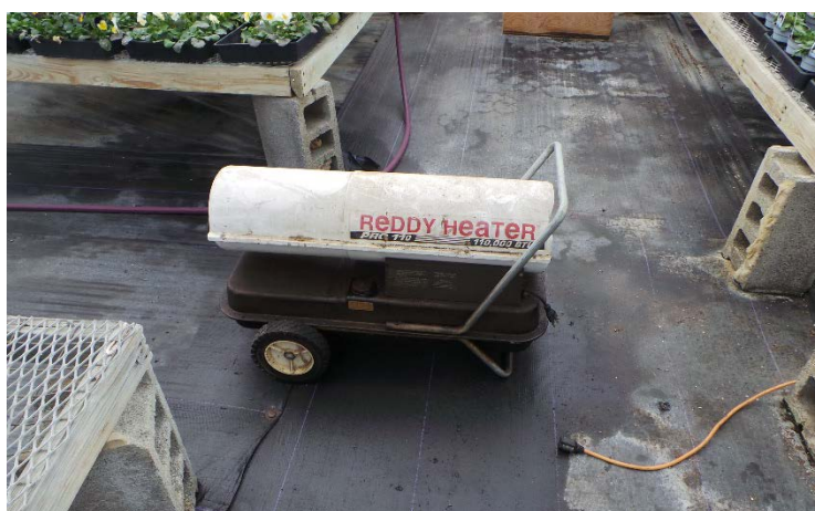
Even the temporary use of unvented heaters on a cold night can create cropping problems in greenhouses and high tunnels. (Photo by Thomas G. Ford)
