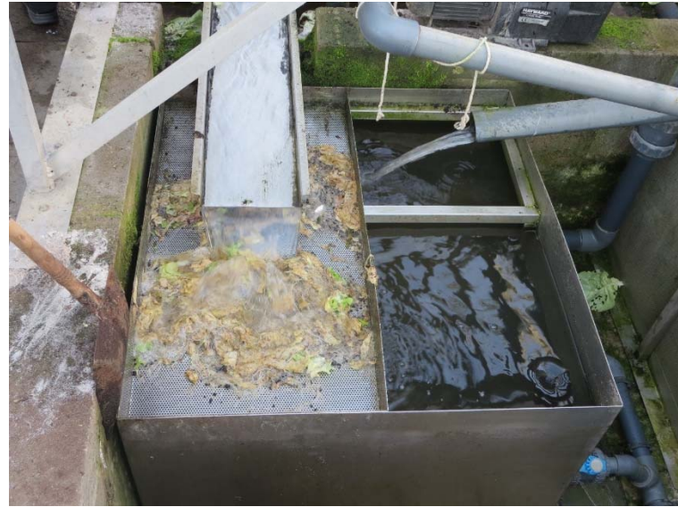
Figure 4. Example of a coarse filter ( >500 \mu\text{m} (35 U.S. mesh)). Coarse filters are used to remove large organic particles such as plant leaves and roots, or large particles of substrate.
