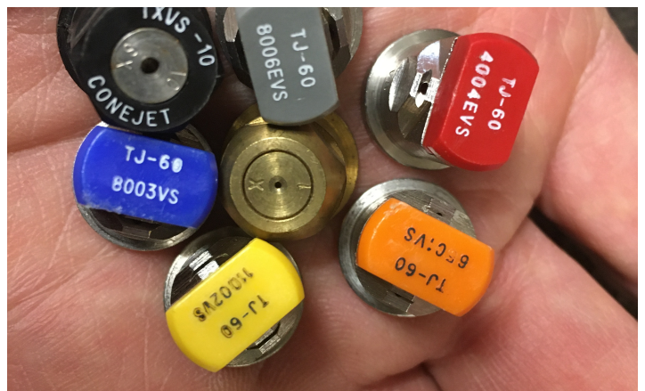
Swapping out nozzles is one simple way to adjust gallonage when making spray applications.
