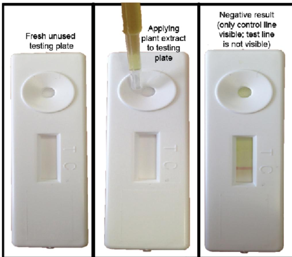
Figure 5. Applying the plant-buffer extracted sample to a test plate, resulting in a negative result (i.e. - no disease detected).
