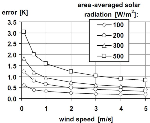
Figure 2. Temperature measurement errors (degrees in Celsius) caused by solar radiation and wind speed around the sensor (Erell et al., 2005; Sensor diameter = 1 mm). 1 degree K = 1 degree C = 1.8 degrees F
