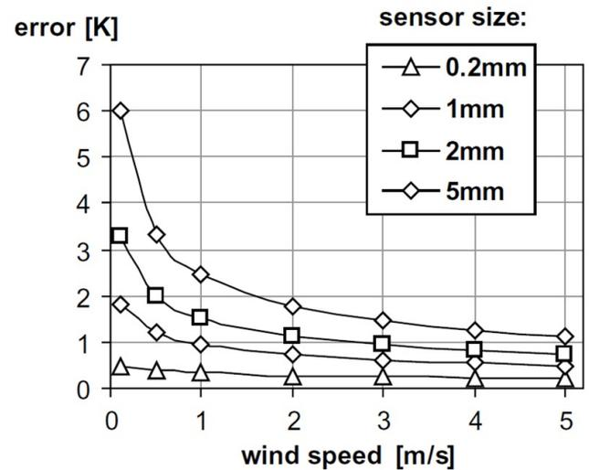
Figure 3. Temperature measurement errors (degrees in Celsius) caused by sensor size and wind speed under 300 W/m<sup>2</sup> solar radiation (Erell et al., 2005). 1 degree K = 1 degree C = 1.8 degrees F
