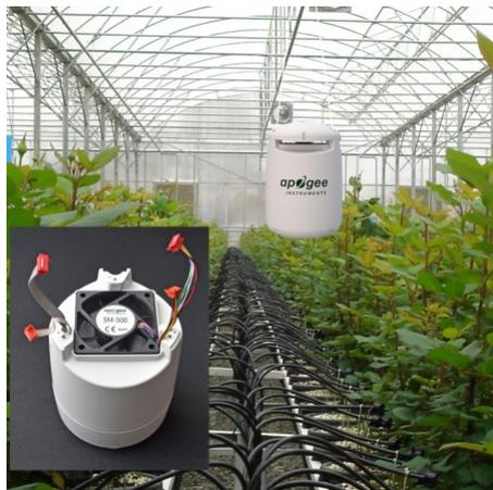
Figure 1. A commercially available aspirated radiation shield used for temperature and humidity measurements under radiation in greenhouse. The shield has reflective material and an aspiration fan (shown in the inserted photo) to bring air to the sensor at a recommended rate for accurate measurement. (Photos by courtesy of Apogee Instruments Inc.)
