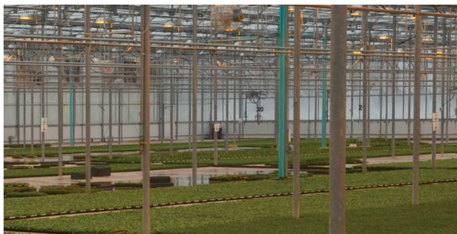
Figure 1. Traditional supplemental lighting of young plants with high-pressure sodium lamps.
