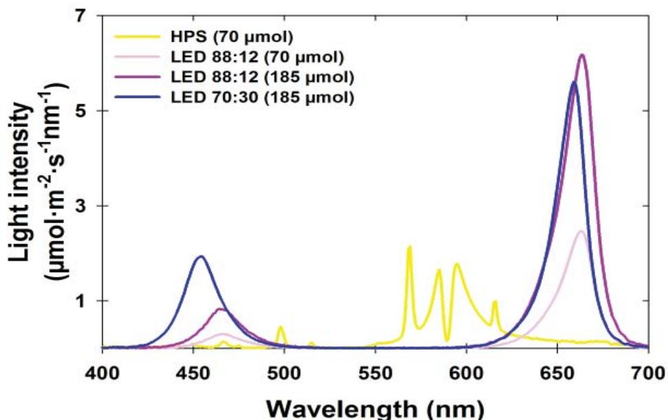
Figure 4. Light quality of high-pressure sodium (HPS) lamps delivering  $70 \mu\text{mol}\cdot\text{m}^{-2}\cdot\text{s}^{-1}$ , light-emitting diodes (LED) delivering 70 or 185  $\mu\text{mol}\cdot\text{m}^{-2}\cdot\text{s}^{-1}$  of (%) 87:13 red:blue light or 185  $\mu\text{mol}\cdot\text{m}^{-2}\cdot\text{s}^{-1}$  of (%) 70:30 red:blue light at canopy level.
