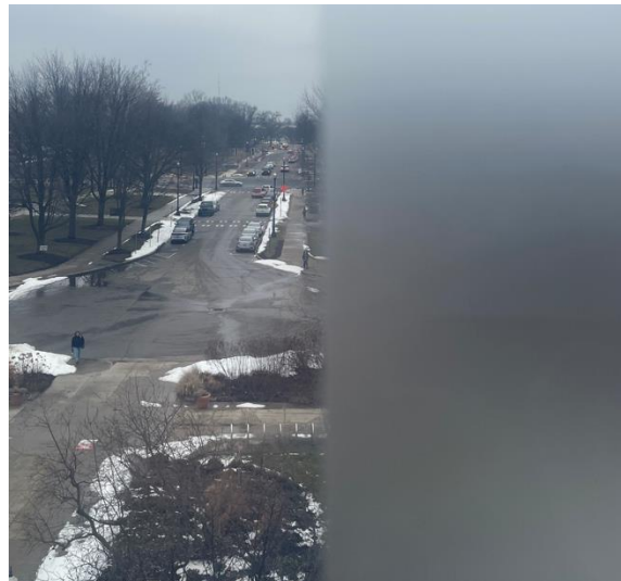
Figure 1. Looking through a diffuse film (right) and a non-diffuse film (left). These films have nearly identical PAR transmission. Photo by C. Kubota.
