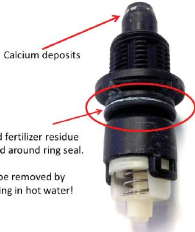
Figure 2. This main piston had an excessive amount of fertilizer, (and maybe fungicide) encrusted in between the seal and the piston, calcium deposits didn't help.
