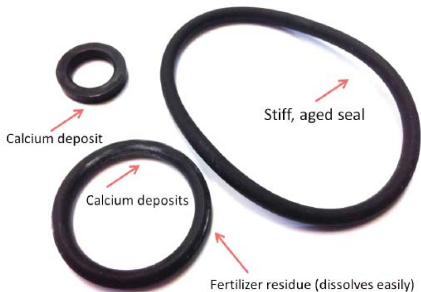
Figure 1. Small issues that have big effects! Calcium deposits and dried fertilizer salts on these seals caused failure, as did the 5 year old, stiff seal seen on right.
