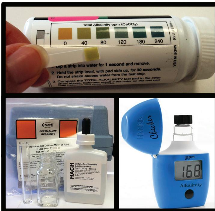
Figure 2. Examples of do-it-yourself testing kits for water alkalinity. Top: A test strip kit that approximates water alkalinity. Bottom Left: A titration style water alkalinity testing kit. Bottom Right: A handheld colorimeter.
