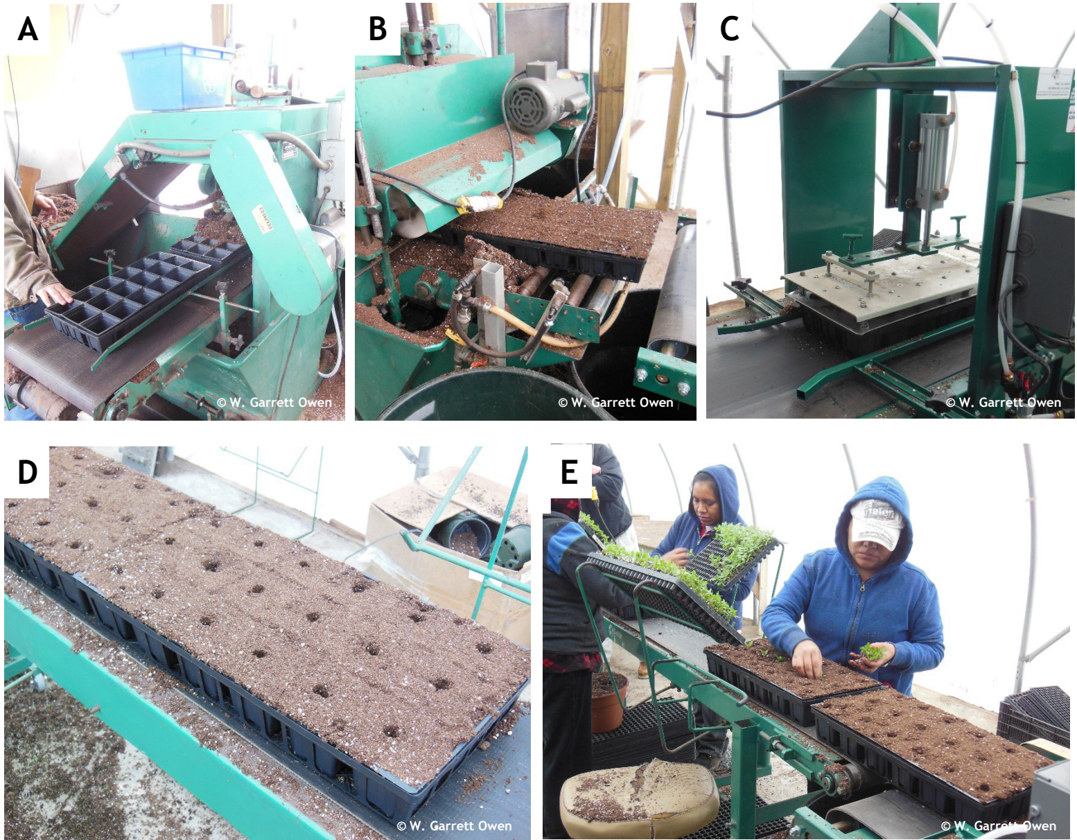
Figure 8. An example of a included a mobile transplanting line designed to improve production efficiency by using (A) a conveyor belt to move flats and insert down the production line to be (B) filled with soilless substrate. Excessive substrate is brushed off the top of the flat to ensure even distribution and mitigate waste. An automatic (C) dibble board presses into the substrate to create (D) transplanting holes that are consistently spaced with a uniform depth. Greenhouse staff can easily and efficiently (E) transplant plugs into the dibbles holes. Photos by: W. Garrett Owen, OSU.
