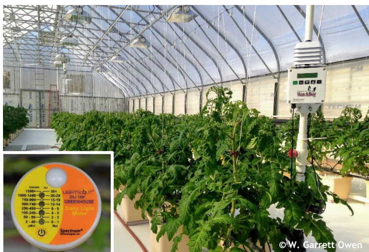
Figure 17. Examples of portable data loggers with light measurement capabilities utilized by greenhouse growers to monitor and manage daily light integral in the greenhouse environment. Photos by: W. Garrett Owen, OSU.
