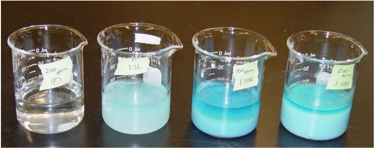
Figure 2. Testing compatibility of 2 different fertilizers using the jar test. The left photos represent the fertilizers mixed at the dilute concentration received by plants (200 ppm N), the subsequent photos L to R represent the two fertilizers mixed at 16x, 100x, and 200x concentration showing they are incompatible in the same stock tank. Photo by N. Mattson, Cornell University.
